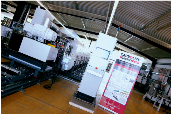
Fig. 3 The fully assembled plant in Carbolite Gero, which can be operated from the front automatically by means of a touch panel
