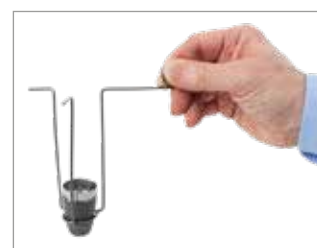
Standard wire crucible holder shown with crucible & lid (VMF/ASTM)
