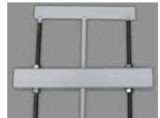
Coal levelling device
