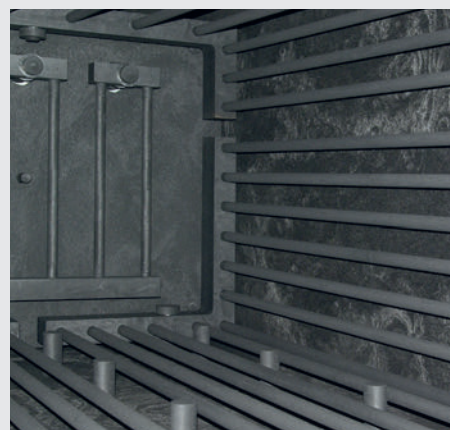
Fig. 20: View into HTK 400 mantle heater with back wall heating and several graphite pillars at the bottom supporting the movable retort for convenient loading and unloading of the furnace
