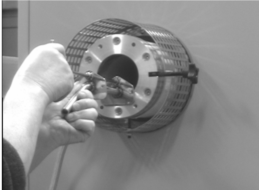
Fig 13c. Loading Samples into the Work Tube
