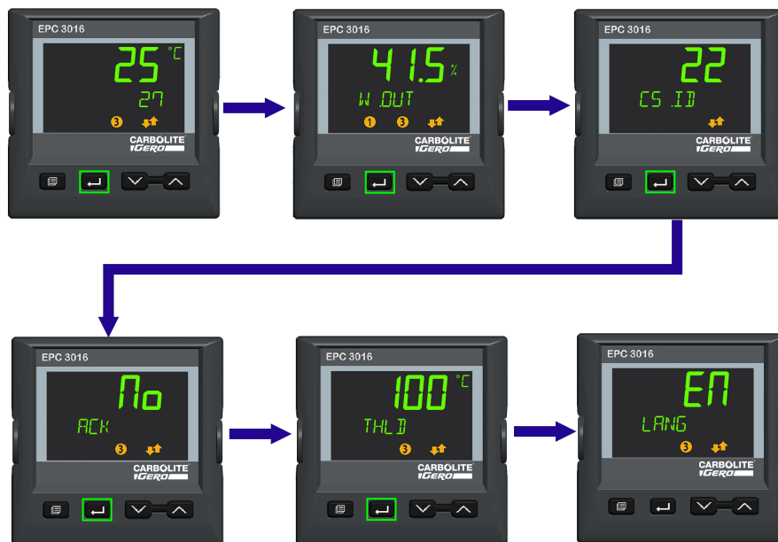
Scrolling through Controller Settings at Operator Level 2
