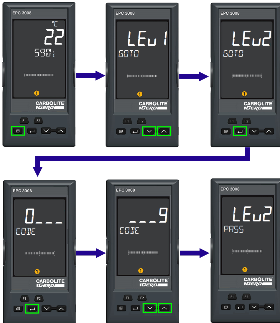
Changing Operator Level to Level 2
