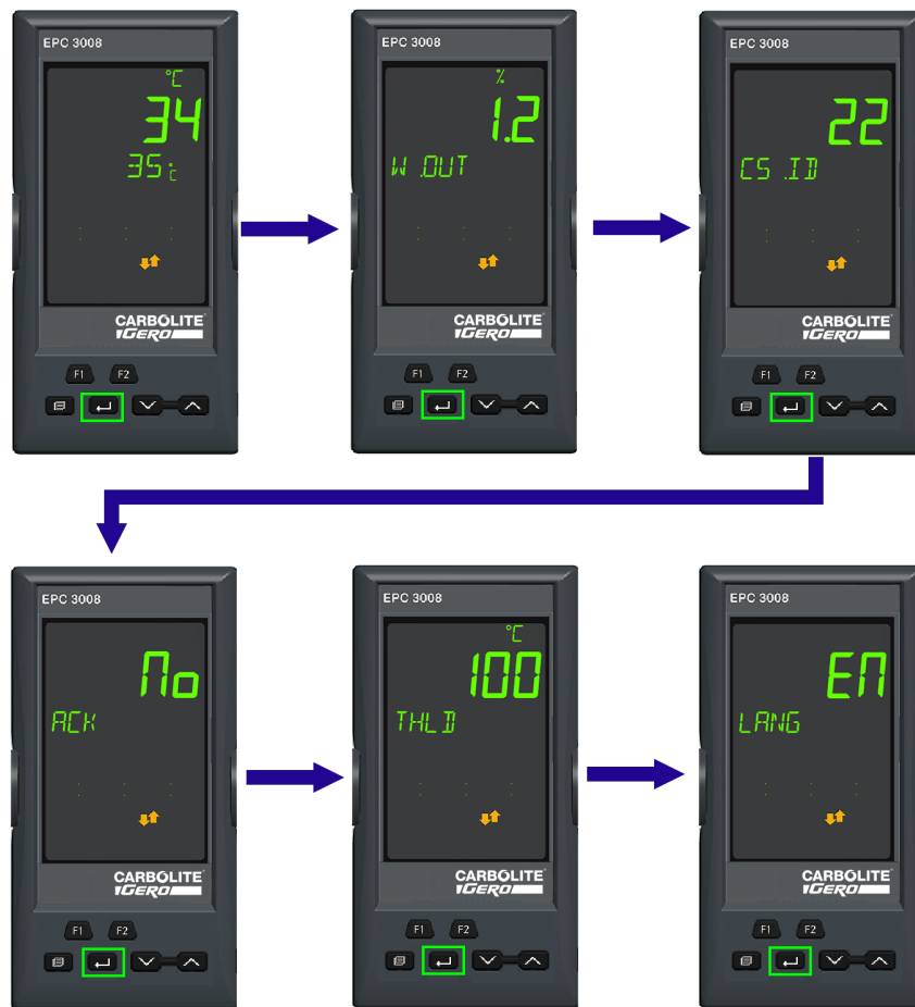
Scrolling through Controller Settings at Operator Level 2
