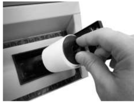
Fig 30 - Squeeze the spindle pins to release printer roll
