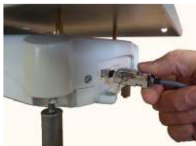
Fig 18 - Connecting the cable to the balance
