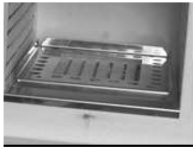
Fig 25 - Balance pan extension in place
