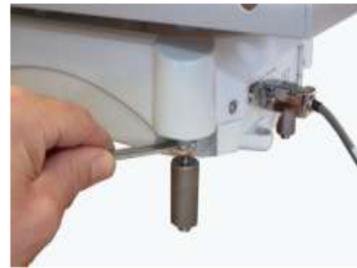
Fig 23 - Using a spanner adjust the legs on the balance until the indicator on the bubble arm shows that it is level
