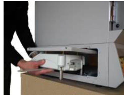
Fig 17 - Partly insert the balance through the left hand opening then connect the cable and earth lead
