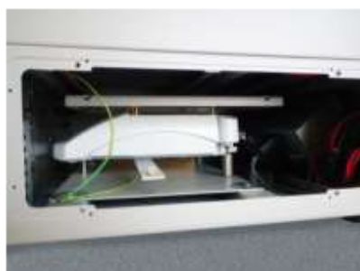
Fig 21 - Insert the balance through the left side with the read of the balance towards the front of the furnace
