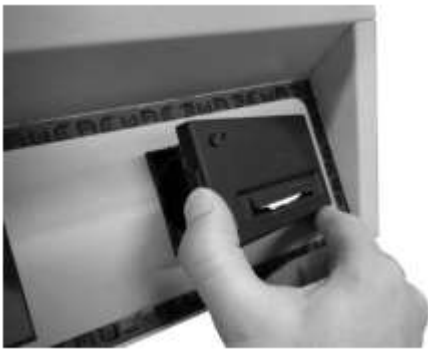
Fig 29 - Release clip and swing open the printer
